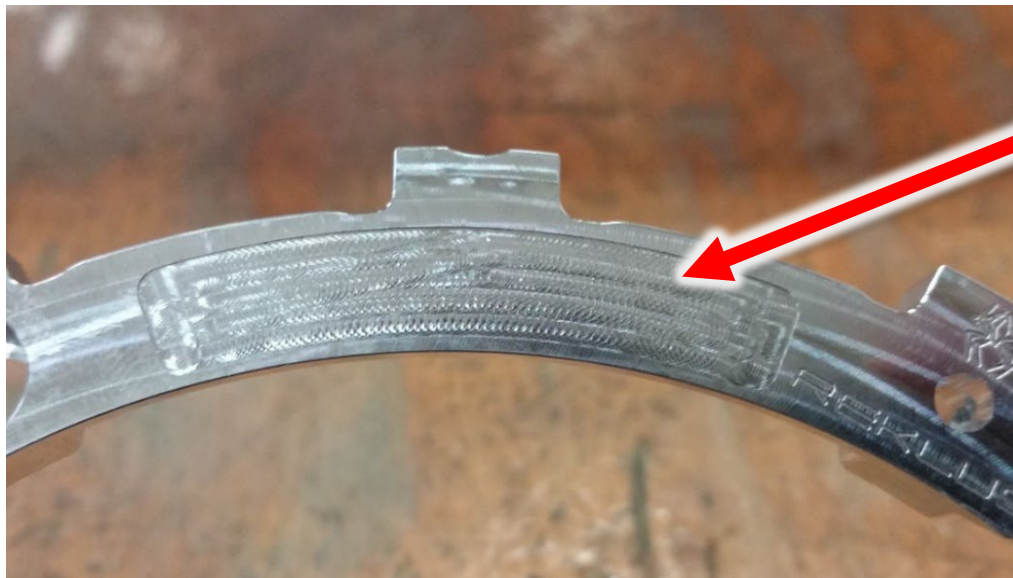
Missing friction pad
